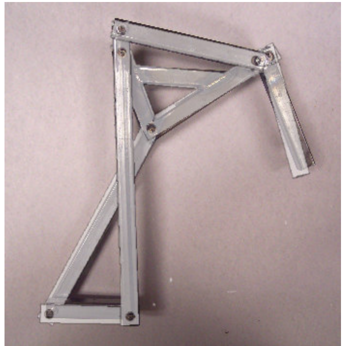
Figure 3. Fabricated major index finger
